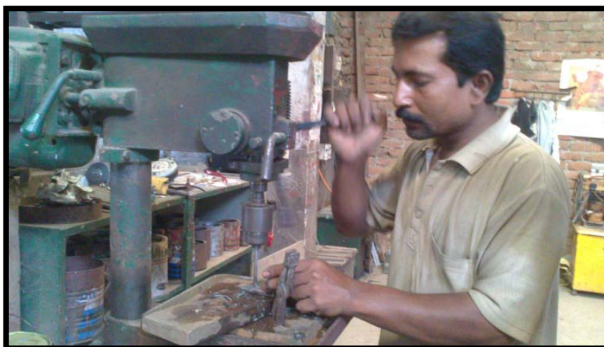
Figure 7-15: The carpenter is drilling holes into the "L" shaped clamp.
