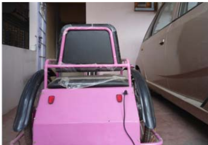
Figure 5.6: Fabrication of rear Guard
