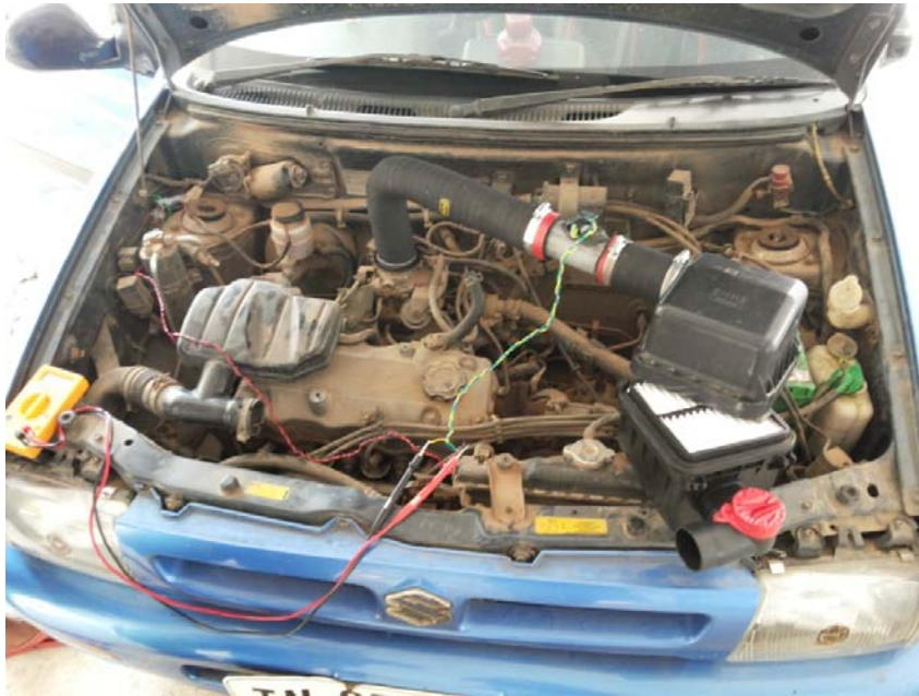
Fig 22: Assembly of the setup over the inlet manifold
